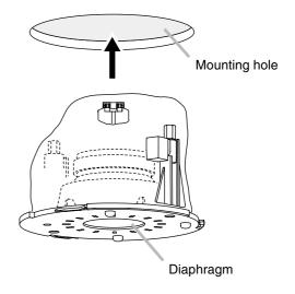
4-2. Rotate and tighten the mounting tab axis screws (2 places) on the unit clockwise to their full stop in order to grip the ceiling panel with the mounting tabs.
